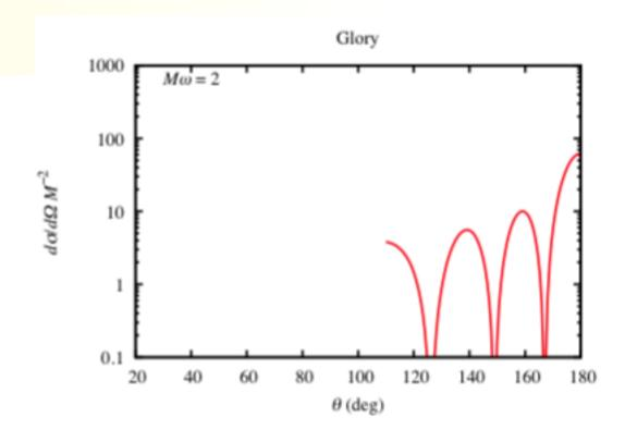
$$\frac{d\sigma_{\rm sc}}{d\Omega} = 2\pi\omega b_g^2 \left| \frac{db}{d\theta} \right|_{\theta=\pi} J_{2s}^2(\omega b_g \sin \theta)$$
